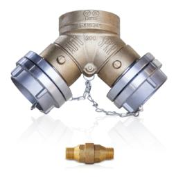
Model AFDC-100 is used as auxiliary connections through which the fire department can pump water to supplement the fire protection water supply. Provides minimum 250 gpm (950 lpm) flow per 21/2" inlet.
